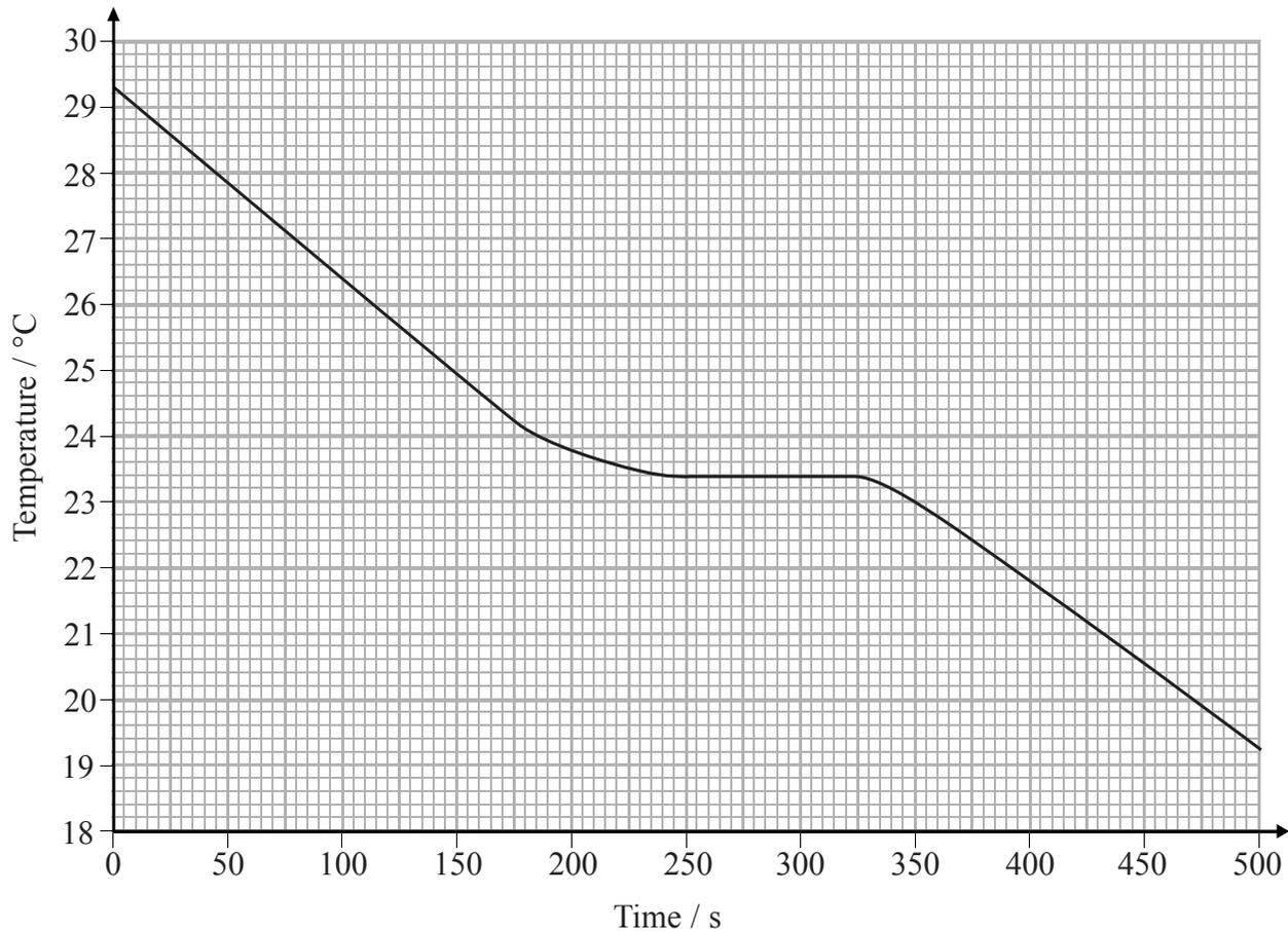
(a) Use the graph to show that the rate at which thermal energy was transferred from the liquid chocolate was about 50 W.
